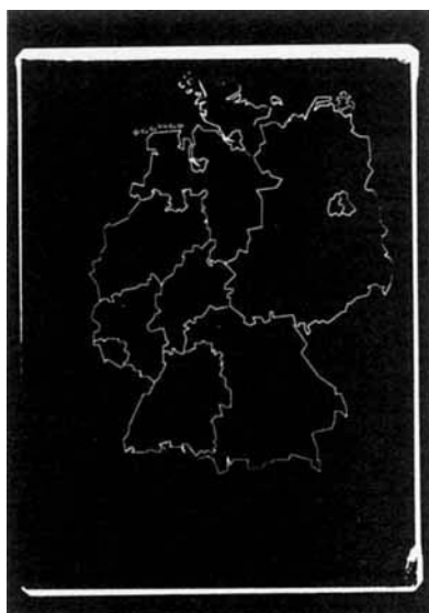
Fig. 9. Outlines of the Federal Republic of Germany and the German Democratic Republic drawn by a Ne-YAG-laser onto a homogeneous aligned nematic LC-homopolymer. Photomicrograph between crossed polarizers and parallel to the orientation of the director. (Cell: 4 cm x 3 cm; thickness: 10 \mu m; line width: 20–30 \mu m, IAF, Freiburg).
